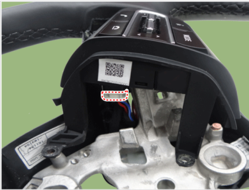
7. Disconnect the connector and then remove the steering wheel body.
